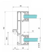
$\bullet$  The double glazed aluminium door frame with integrated hinge & receiver profile is suitable for glass door thicknesses of 8-10mm and 8 - 12.76mm thick fixed panels.
