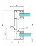
• The double glazed aluminium door frame with integrated hinge & receiver profile is suitable for glass door thicknesses of 8-10mm and 8 - 12.76mm thick fixed panels.
