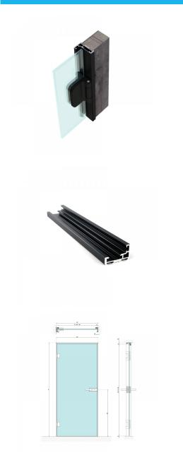
• The L-type aluminium door frame with integrated hinge & receiver profile is suitable for glass thicknesses of 8-10mm. The recommended max door height is 2400mm. Above a height of 2200 mm, it is recommended to use 3 hinges.
