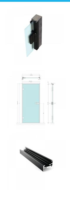
• The Z-type aluminium door frame with integrated hinge & receiver profile is suitable for glass thicknesses of 8-10mm. The recommended max door height is 2400mm. Above a height of 2200 mm, it is recommended to use 3 hinges.
