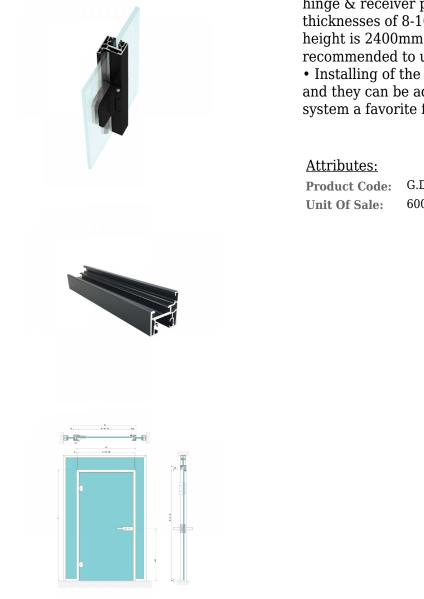
45 9 9 44 31 • The H-type aluminium door frame with integrated hinge & receiver profile is suitable for glass thicknesses of 8-10mm. The recommended max door height is 2400mm. Above a height of 2200 mm, it is recommended to use 3 hinges.
