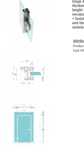
• The H-type aluminium door frame with integrated hinge & receiver profile is suitable for glass thicknesses of 8-10mm. The recommended max door height is 2400mm. Above a height of 2200 mm, it is recommended to use 3 hinges.
