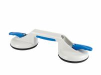
The Veribor® 2-cup suction lifter has a large, non-slip gripping area and lies perfectly in your hand. The levers have an ergonomic and user-friendly design. Their wide surface enables optimum force absorption. They are dimensionally stable but still soft enough to adapt to the surface during vacuum generation. The 2-cup suction lifter is suited for loads of up to 50 kg (two-fold safety factor) and can be used for all materials and objects with gastight surfaces.
