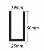
These U-Channels provide the most economical way to glaze heavy glass. Using the Deep U-Channel on the top and Shallow U-Channel on the bottom allows for the 'shuffle glaze' method of glazing. The glass can be secured with silicone sealant or our Top Load Roll-In Glazing Gasket. Roll in wedge gaskets for 10 or 12mm glass are sold separately.
