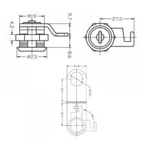
Cabinet swing glass door lock for double doors for glass thickness 5-6mm. Accessories:
