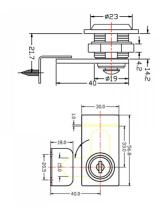
Cabinet swinging glass door lock for double door for glass thickness 5-7mm.
