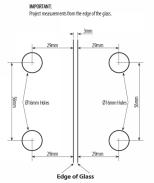
Door swings 180° out only. Suitable for 6mm to 8mm thick toughened glass.
