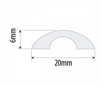
Mounted directly below the shower door to let the water drain back into the shower stall.
