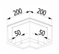
$\bullet$  Suitable for line loads up to 3kN in accordance with BS6180.
