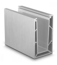
Ideal small and slim system for mounting on to the side of a parapet wall to increase the height of it up to 1100mm high and achieve suitable barrier loads of up to 0.74kn with the correct glass selection. Can also be used to fix to the side of a full height wall to act as an additional windbreak without losing the views that a wall would result in.
