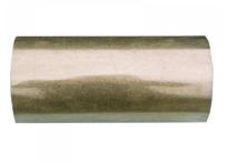
60 micron clear safety backing film, is a high tack biaxially orientated polypropylene film, which is fully tested to BS EN 12600 and class 2B2 for frontal impact. For use on all sizes of mirror and can be applied by automatic laminator or manually.
