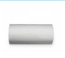
60 micron white safety backing film, is a high tack biaxially orientated polypropylene film, which is fully tested to BS EN 12600 and class 2B2 for frontal impact. For use on all sizes of mirror and can be applied by automatic laminator or manually.
