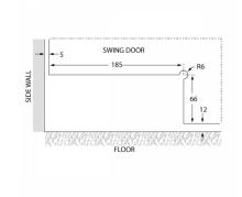
Bottom patch fitting with concealed spring for door closing. With this fitting there is now no need to dig out for traditional floor spring boxes especially in areas where underground services may be present such as underfloor heating. These are ideal for offices, internal doors or external doors that may be sheltered from extreme wind.
