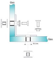
It consists of turned articles and screws in stainless steel AISI 316L to fix the angle bracket with L-junction between glass and glass.
