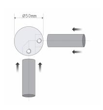
The joint is made of stainless stell AISI 303 allowing the quick junction at 90 degrees of two tubes.
