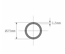
The upper rail is made of stainless steel AISI 316L and is available in 3 mtr length tubes.
