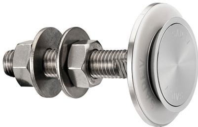
Fixed bolt with a countersunk head for use in spider glazing systems. Manufactured using 316 grade stainless steel. Standard 65mm long axis and suitable for 22 - 26mm thick glass. Please see the other bolts in the range for additional glass thicknesses. Special dimension glass bolts available on request. Glassparts recommend using thread locking compound whenever possible. These items are not held in stock and will require approximately 1-2 weeks delivery time
