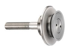
Fixed bolt with a countersunk head for use in spider glazing systems. Suitable for glazing from the outside or blind access glazing. Manufactured using 316 grade stainless steel. Standard 66mm long axis and suitable for 22 - 26mm thick glass. Please see the other bolts in the range for additional glass thicknesses. Special dimension glass bolts available on request. Glassparts recommend using thread locking compound whenever possible.
