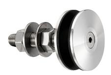
Fixed bolt with a 60mm diameter flat head for use in spider glazing systems. Suitable for glazing from the outside or blind access glazing. Manufactured using 316 grade stainless steel. Standard 65mm long axis and suitable for 8 - 15mm thick glass. Please see the other bolts in the range for additional glass thicknesses. Special dimension glass bolts available on request. Glassparts recommend using thread locking compound whenever possible.
