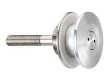
Fixed bolt with a 60mm diameter flat head for use in spider glazing systems. Suitable for glazing from the outside or blind access glazing. Manufactured using 316 grade stainless steel. Standard 66mm long axis and suitable for 8 -15mm thick glass. Please see the other bolts in the range for additional glass thickness'. Special dimension glass bolts available on request. Glassparts recommend using thread locking compound whenever possible. These items are not held in stock and will require
