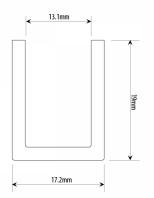
U channel suitable for 12mm thick glass.
