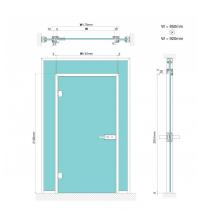
Grey Anodised Standard Door Frame Kit pre cut to size to suit a  $850 \text{mm} \times 2057 \text{mm}$  door leaf.
