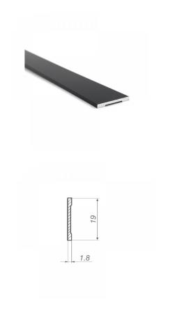
Create a Crittall Style glass partition using this flat aluminium black profile. Cut to the desired length and apply a clear acrylic tape 0.75mm thick such as H.A7200.09.07 to stick it to the glass.
